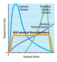
1. Hydraulic Dashpot (High stopping force at start of the stroke).
