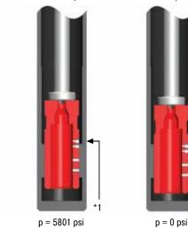
\* The load velocity reduces continously as you travel through the stroke due to the reduction in the number of metering orifices (\*) in action. The internal pressure remains essentially constant and thus the force vs. stroke curve remains linear
