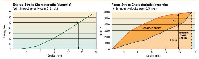
With the aid of the characteristic curves above you can estimate the proportion of the total energy that will be absorbed. Example: With impact energy of 50 Nm the Energy-Stroke diagram shows that a stroke of about 14 mm is needed. On the Force-Stroke diagram you can estimate the proportion of absorbed energy to rebound energy at this stroke length.
