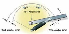
It is possible to use only one shock absorber for both end positions by using different pivot points as shown.
