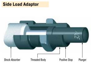
With side load impact angles of more than 3° the operation lifetime of the shock absorber reduces rapidly due to increased wear of the rod bearings. The optional side load adaptor provides long lasting solution. Secure the side load adaptor with Loctite or lock nut on the shock absorber.
