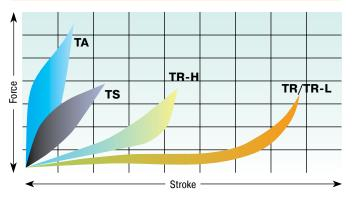
Characteristics of dynamic energy absorption for impact velocity over 1.64 ft/sec. For impact velocities under 1.64 ft/sec, please request a static characteristic curve.
