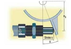
Soft end-of-travel damping on rotary movements
