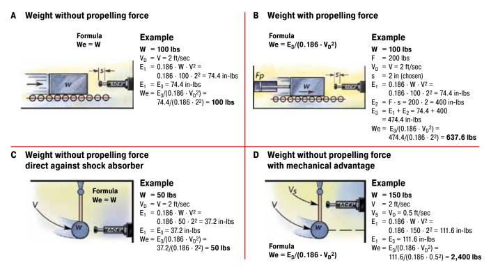
The effective weight (We) can either be the same as the actual weight (examples A and C), or it can be an imaginary weight representing a combination of the propelling force or lever action plus the actual weight (examples B and D).
