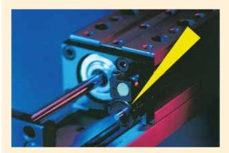
Miniature shock absorber in linear pneumatic module
