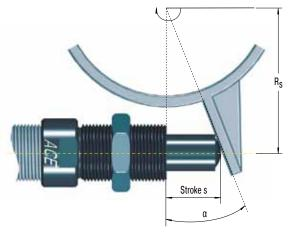
**Problem:** Rotating impact motion causes high side load forces on the piston rod. This increases bearing wear and possibly results in rod breakage or bending. **Solution:** Install side load adaptor.
