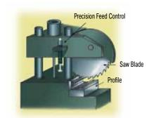
Varying material types, hardness and wear on the saw blade causes the cutting pressure to vary greatly. However the saw advance speed should remain constant as changes cause breakage of the material being cut or of the saw blade.
