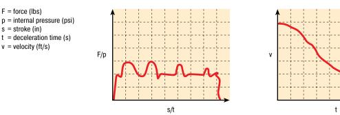
ACE shock absorbers provide linear deceleration and are therefore superior to other kinds of damping elements. It is easy to calculate around 90% of applications knowing only the following 5 parameters:
