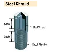
Grinding beads, sand, welding splatter, paints and adhesives etc. can adhere to the piston rod. They then damage the rod seals and the shock absorber quickly fails. In many cases the installation of the optional steel shroud can provide worthwhile protection and increase lifetime.
