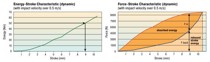
With the aid of the characteristic curves above you can estimate the proportion of the total energy that will be absorbed. Example: With impact energy of 50 Nm the Energy-Stroke diagram shows that a stroke of about 8.8 mm is needed. On the Force-Stroke diagram you can estimate the proportion of absorbed energy to rebound energy at this stroke length.
