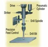
A high force is necessary at the start of drilling when the drill first contacts the sheet. After the initial cut this high force causes the drill to break through. This results in jagged edges rather than a smooth clean hole and also causes tool breakage.
