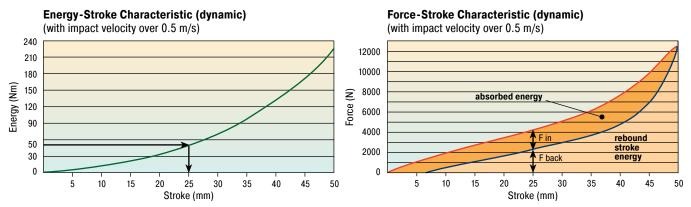
With the aid of the characteristic curves above you can estimate the proportion of the total energy that will be absorbed. Example: With impact energy of 50 Nm the Energy-Stroke diagram shows that a stroke of about 25 mm is needed. On the Force-Stroke diagram you can estimate the proportion of absorbed energy to rebound energy at this stroke length.
