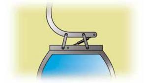
Swinging movements cushioned by hydraulic dampers
