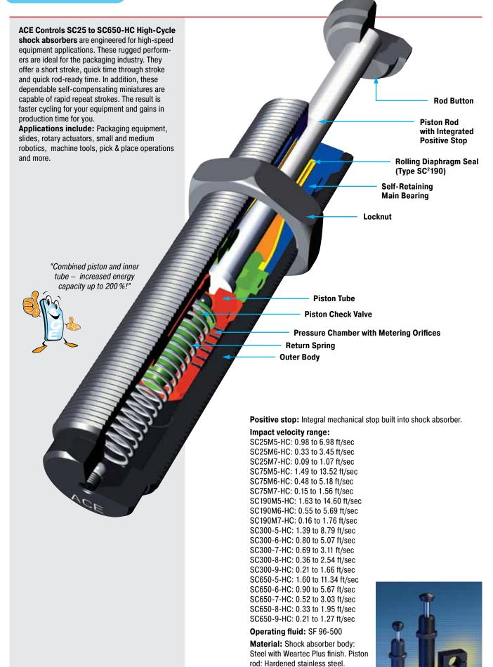
**Mounting:** In any position. If precise end position is required, consider use of the optional stop collar. **Operating temperature range:**
