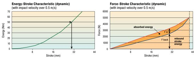
With the aid of the characteristic curves above you can estimate the proportion of the total energy that will be absorbed. Example: With impact energy of 50 Nm the Energy-Stroke diagram shows that a stroke of about 31 mm is needed. On the Force-Stroke diagram you can estimate the proportion of absorbed energy to rebound energy at this stroke length.
