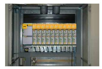
AC890 air ducting components make easy work of cabinet building when force ventilation is to be used. The exhaust duct, supplied in 1 meter sections, is mounted to the top of the AC890 heatsinks and includes a 190 CFM fan. This arrangement provides a very effective means of cooling by drawing air directly through the drives' heat sinks and out of the air outlets which can be flex-ducted out of the cabinet. See part numbers in table to right.
