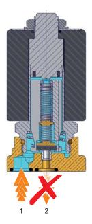
Coil energized, Plunger in the open position, Full flow.
