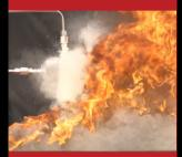
The **AFEX** nozzle delivers a conical discharge pattern for broad distribution of the dry chemical agent, creating a "total flooding" system and maximizing area coverage.
