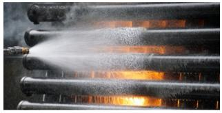
Liquid agent fire suppression systems provide exceptional cooling abilities to suppress Class A (debris) and Class B (fuel) fires. The liquid agent works by cooling hot surfaces, separating fuel hydrocarbon molecules to prevent fire reignition and form a layer of foam to suffocate flames. Liquid systems are especially designed to protect high risk vehicle components, such as turbochargers, exhaust components, and Tier 4 aftertreatment components.
