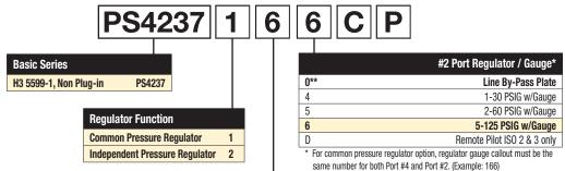
\*\* Pressure line by-pass option can only be used with independent pressure regulators.
