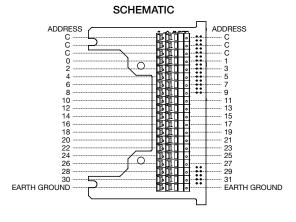
All commons internally connected on terminal strip
