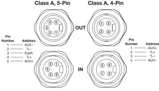
\* 7/8" logic power has no connection to internal P2H unit but does carryover to OUT 7/8" connector (for jumper logic power only). Logic power for P2H unit will be supplied from M12 (pin 1 & 3).
