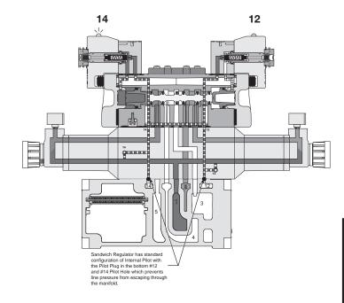
When using an Independent Pressure Sandwich Regulator, the cylinder outlet ports are reversed. The 12 end energizes the #4 port and the 14 end energizes the #2 port. The 3-Position CE and PC functions are also reversed. Do not use with Sandwich Flow Controls. Independent Port Sandwich Port Regulators combine the #3 and #5 valve exhaust ports into the #5 exhaust at the manifold/subbase interface. The #3 port flow control will control both #3 and #5 exhaust. #5 port flow control is ineffective.
