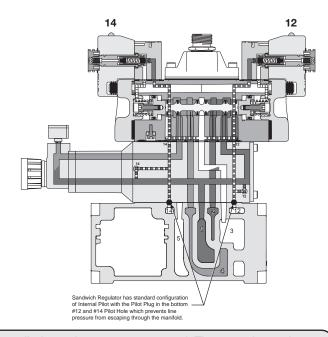
When using an Independent Pressure Sandwich Regulator, the cylinder outlet ports are reversed. The 12 end energizes the #4 port and the 14 end energizes the #2 port. The 3-Position CE and PC functions are also reversed. Do not use with Sandwich Flow Controls. Independent Port Sandwich Port Regulators combine the #3 and #5 valve exhaust ports into the #5 exhaust at the manifold/subbase interface. The #3 port flow control will control both #3 and #5 exhaust. #5 port flow control is ineffective.
