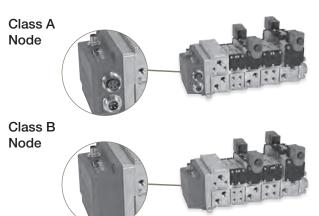
The Class A node has (1) 3 pin M12 connector for communication and logic power from any class A IO-Link master, and (2) 7/8" connectors for auxiliary valve power IN and OUT.
