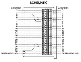
All commons internally connected on terminal strip
