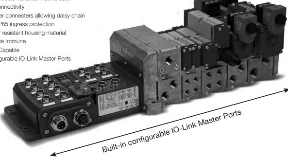
The PCH Network Portal redefines and revolutionizes decentralized machine I/O's architecture. The PCH Network Portal was engineered to support industrial ethernet protocols and the open protocol IO-Link with configurable inputs/outputs with true PNP/ NPN circuitry switching on each port for easy machine design changes. This integrated configurability gives the user flexibility in designing custom I/O architecture on the fly.
