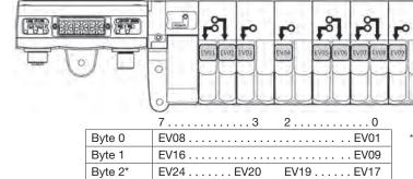
Byte 2 / Bits 3 to 7 are only available when connected to H Series Micro or H Series ISO valve manifolds. The Moduflex valve series is limited to 19.
