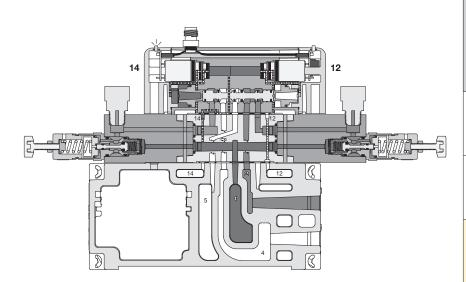
When using an Independent Pressure Sandwich Regulator, the cylinder outlet ports are reversed. The 12 end energizes the #4 port and the 14 end energizes the #2 port. The 3-Position CE and PC functions are also reversed. Do not use with Sandwich Flow Controls. Independent Port Sandwich Port Regulators combine the #3 and #5 valve exhaust ports into the #5 exhaust at the manifold/subbase interface. The #3 port flow control will control both #3 and #5 exhaust. #5 port flow control is ineffective.
