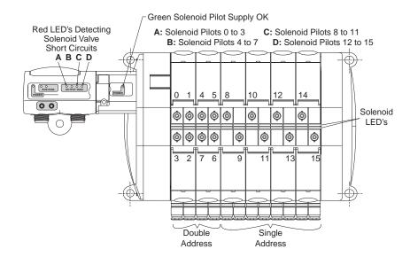
Inside the communication module, solenoid valve control is protected against short-circuits with the following visual indication provided:
