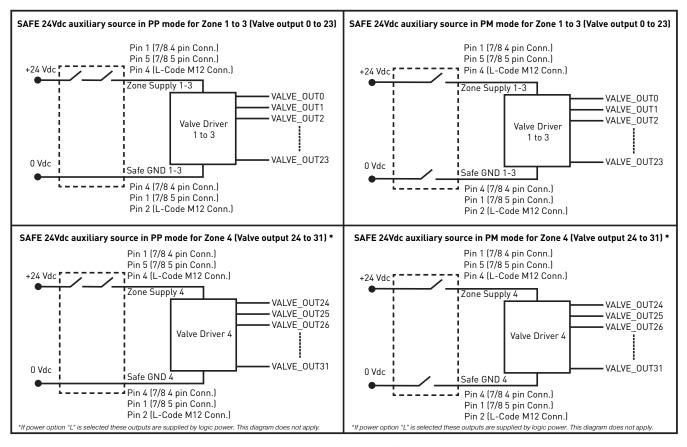
Note: Please check max. power available from the source. Refer to the "Auxiliary power consumption calculation" section.
