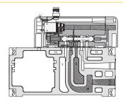
15407-1 18mm Single Solenoid Internal Pilot Manifold Mounted
