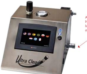
Air supply for Hand Held Launcher located on right side of control station
